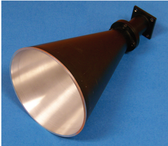
Figure 13.25 Photo of an X-band commercial conical horn ( L = 7.147\lambda , 2\psi_c = 35^\circ ).
